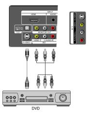
**Note:** If your AV device has both Video OUT terminal and S-Video OUT terminal, S-Video connection is recommended for better picture quality.
